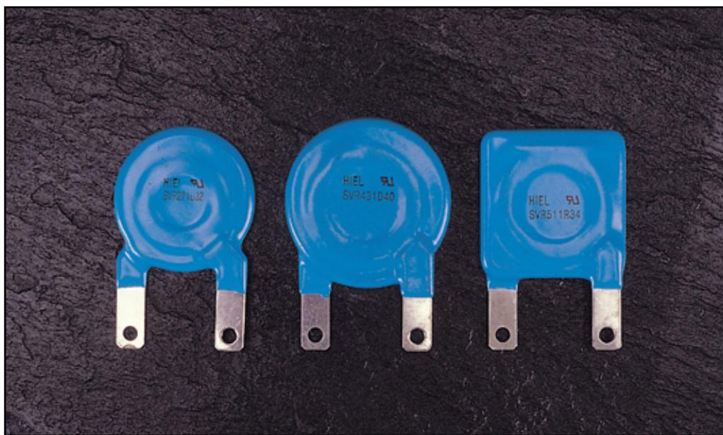
Tap-leaded type of SVR varistor is a heavy duty type with very unique tap terminals which have mounting legs as well as electrical connecting terminals. Tap-leaded type of "SVR" can be adapted in the application of power supplies or transient voltage surge suppressor units where considerably large of surge current or energy absorbtion is required.
