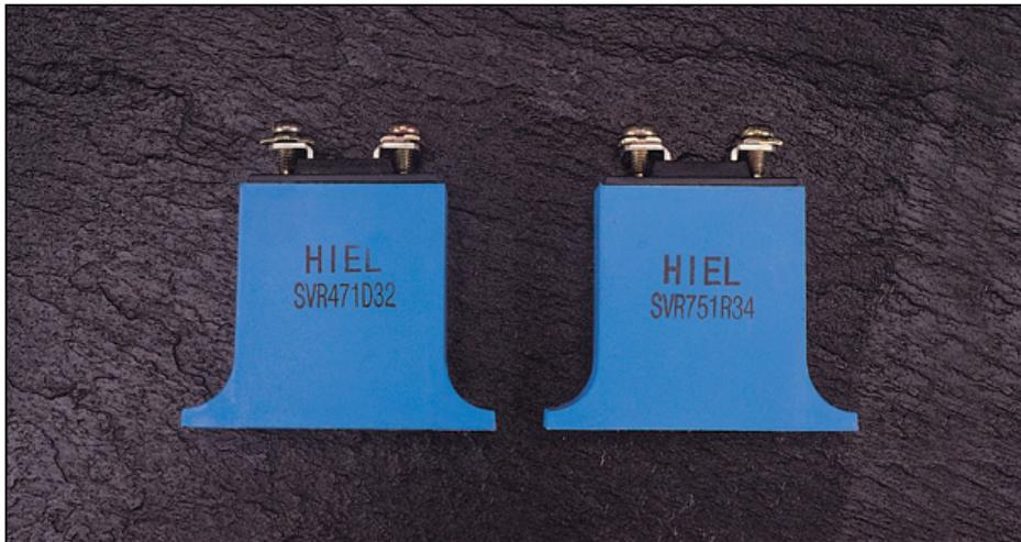
Case type of SVR varistor is defined as cased type of varistor which is assembled into the case, and it has larger capability in surge energy than S and U-series, in the applications of electronic equipments or semiconductor devices from switching and induced lightning surges.
