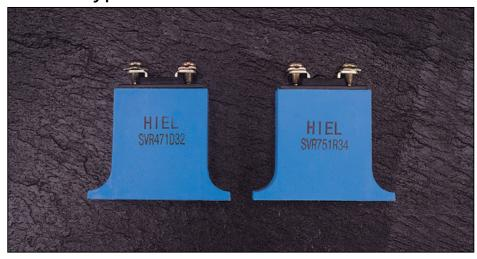
Case type of SVR varistor is defined as cased type of varistor which is assembled into the case, and it has larger capability in surge energy than S and U-series, in the applications of electronic equipments or semiconductor devices from switching and induced lightning surges.
